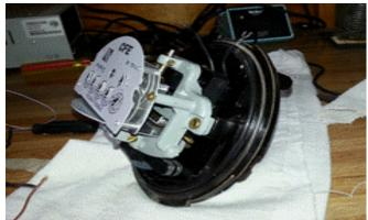
**FIGURE 6.** Traditional household electricity AC energy meter with its front cover removed.
