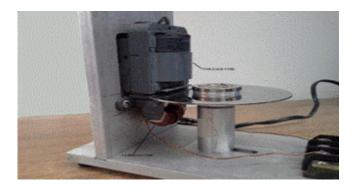
FIGURE 8. Homemade electromagnetic disk induction energy direction sensor.
