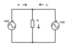
**FIGURE 2.** AC power supplies connected in parallel sharing a load. The current arrows are for reference.
