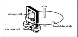
FIGURE 7. Electromagnetic induction disk meter outline.
