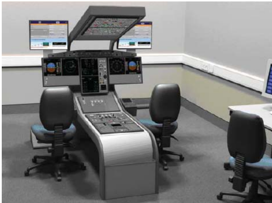
Figure 1. Flight Training Device (FSTD). Source-The impact of flight simulation in aerospace-Royal Aeronautical Society Flight Simulator Group, March 2009.
