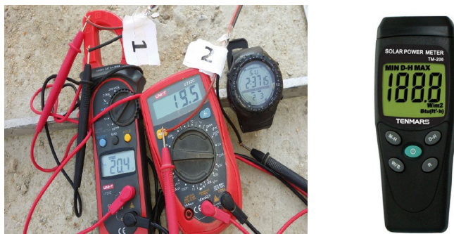
Figure 3. Digital Clamp Meter and Solar Power Meter.
