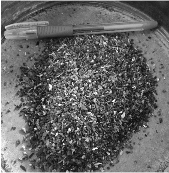
Figure 3. Particles of EWA retained in the sieving process, where the presence of charcoal can be noted. Source: Authors.
