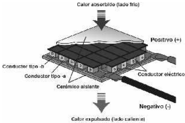
Figure 7. Internal structure of a Peltier cell. Source: Meca Meca and Jiménez Calvo [29].
