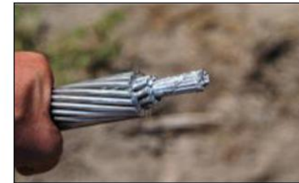
Metallic Composite Core
