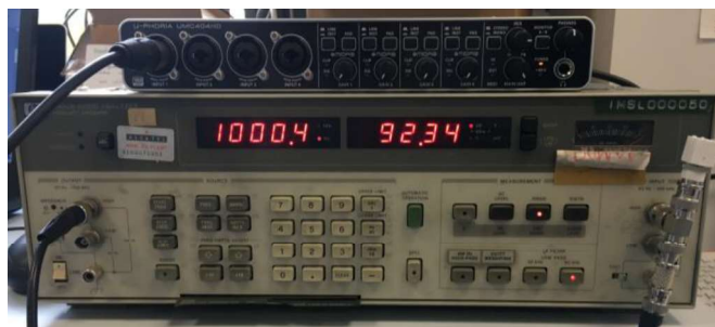
Fig. 2. Profiling the measurement equipment Behringer UMC404HD using a calibrated reference: HP 5903B Audio Analyzer.
