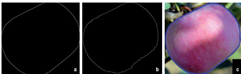
Figure 5. Comparison of the convex hull and contour of an apple. (a) Convex hull of the apple. (b) Edge of the apple extracted using the Canny algorithm. (c) Convex hull of the apple illustrated in the original image.
