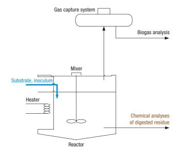
Figure 1. Design of laboratory biogas plant used for biogas for production.
