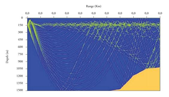
Fig. 2. Underwater sound propagation paths obtained from an acoustic propagation model
