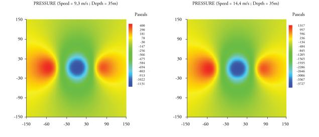
Fig. 5. EShip's Pressure Signature Simulation
