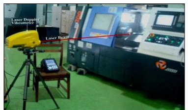
Figure 6 :Measurement of rotating work piece vibration using LDV Source: Venkatarao, Murthy and Mohanrao (2014)
