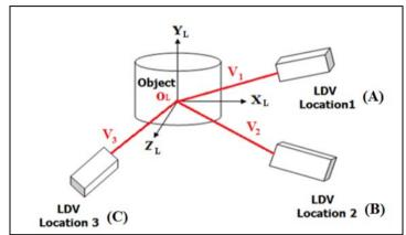
Figure 8: Vibration measurement at arbitrary point on object from three different locations Source: Dongkyu, Hajun, Hossam, Jongsuh, Semyung and Kyihwan (2014)
