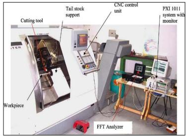
Figure 3: Vibration measurement using accelerometers Source: Chelladurai, Jain, and Vyas (2008)
