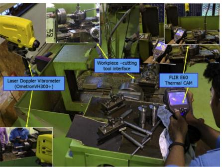
Figure 2:.Experimental test setup in central machine shop Source: Prasad, Sarcar and Satish (2010)
