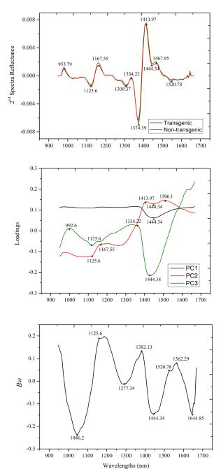
**Figure 4.** Distribution of sensitive wavelengths of transgenic and non-transgenic maize leaves selected by  $2^{nd}$  derivative, PCA-loadings and *Bw*.
