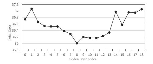
Figure 2: The optimal Neural Network for different hidden layer nodes
