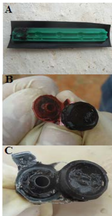
Figure 3. Drip emitters with biofilm: G1 (A), G2 (B) and G3 (C). Source: The authors
