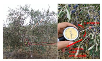
**Figure 1.** Dynamometer with modified hook for make stalk twisting before fruit detachment force (FDF) measurement
