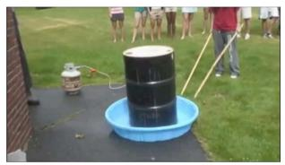
FIGURE 2. Sealed steel barrel filled with water vapor in icy water.
