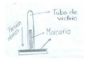
**FIGURE 8.** A schematic presentation of Torricelli experiment (Presión atmos. = atmospheric pressure; Tubo de vidrio = glass tube; Mercurio = mercury).
