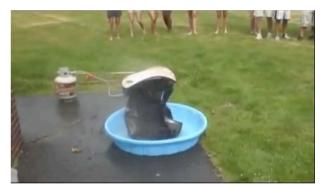
**FIGURE 3.** Steel barrel becomes crushed when the its interior pressure of water vapor becomes very small due to condensation.
