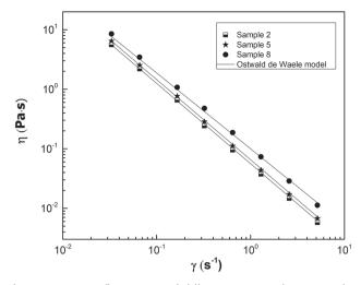
Figure 1. Viscous flow curves of different O/W emulsions samples at room temperature (25 °C). The solid lines represent adjusting to Ostwald de Waele model. Source: Authors
