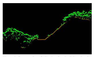
Figure 3. Cross section of LiDAR point cloud data showing three tops (green points) and the ground surface (yellow points).
