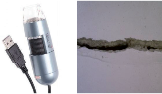
Figure 16. Digital microscopy lens – typical crack image 60 x.
