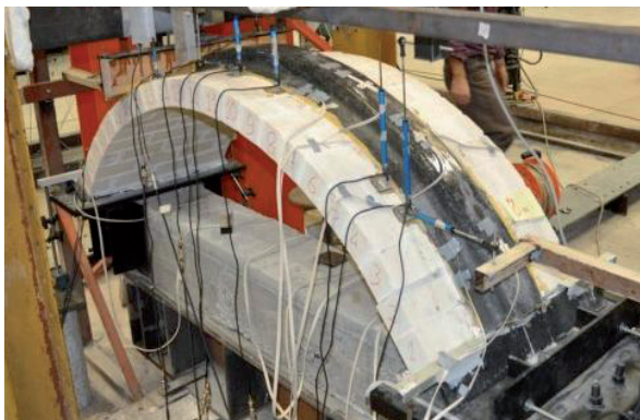
Figure 7. Experimental set-up for the \Omega -WRAP-reinforced vaults.
