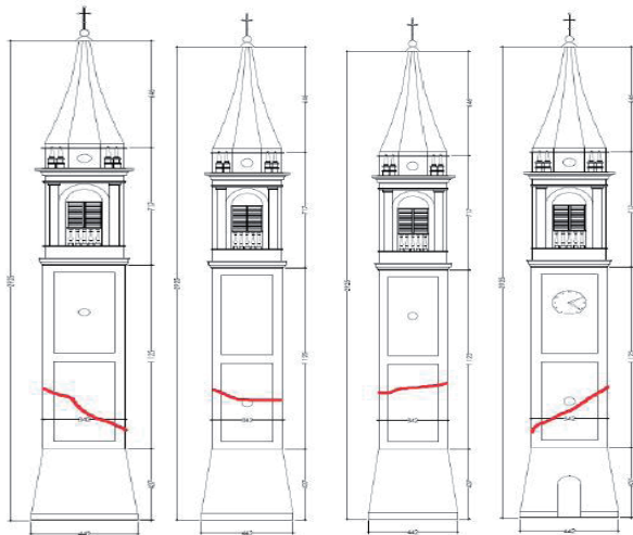
Figure 9. Propagation of crack due to bending.
