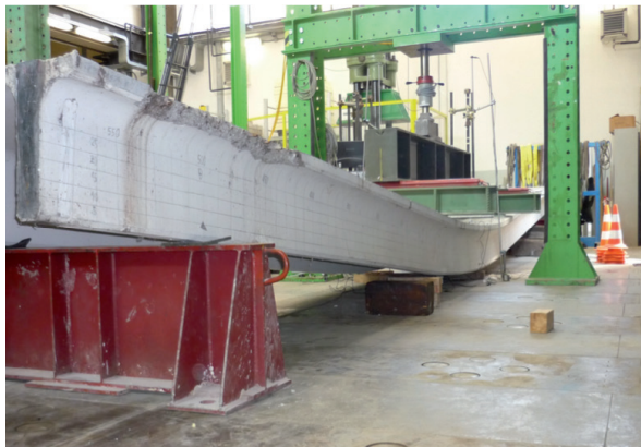
Figure 5. Failure of the control unstrengthened TT beam.
