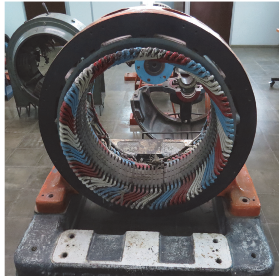
Figure 1. Stator of the electrical machine of 210 kVA. Source: The authors.
