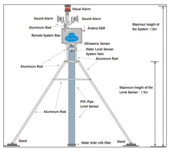
Figure 5: Side view of Nimbusdoid equipment Source: Elaborated for the authors (2016)
