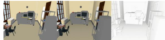
Figure 6. AGAL shader output for ambient occlusion and for edge detection. Rendering of interior of a room. Left: scene texture (no lights!); Center: scene texture and our filter (AO+edges); Right: raw output of our filter.
