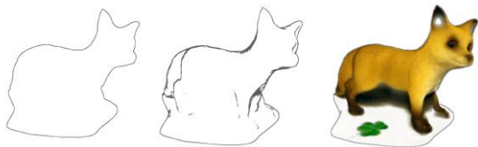
Figure 4. AGAL shader output for purposes of the edge detection. Left: show just the outline of the model, range=2000; Center: show the outline and other inner features of the model, range=1000; Right: result of the shader work – the scene texture is mixed with contours.
