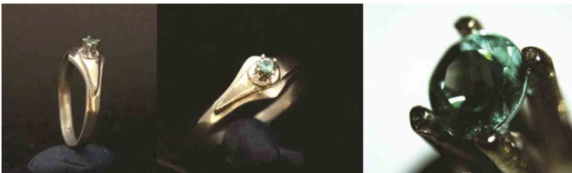
FIG. 10. Photographs of a ring fabricated using investment micro-casting of pre-set emeralds in the chamotte/plaster refractory mold developed in the present study.
