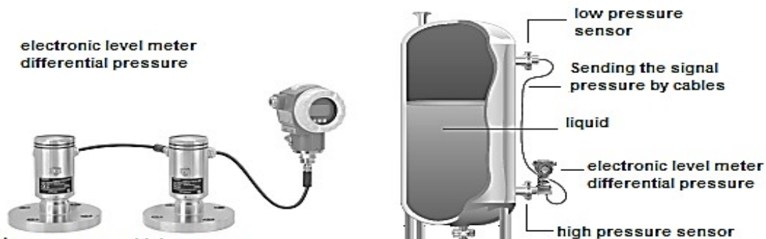
Figure 4. Level Meter electronic differential pressure in a closed container. Source: [25], [27]
