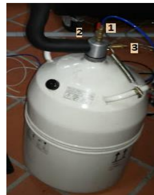
Figure 6. Storage tank of LN2 and its respective valve 1) air intake, 2) nitrogen gas exit, 3) escape valve.
