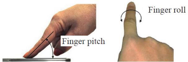
Figure 3. Illustration of the finger pitch and the finger roll.
