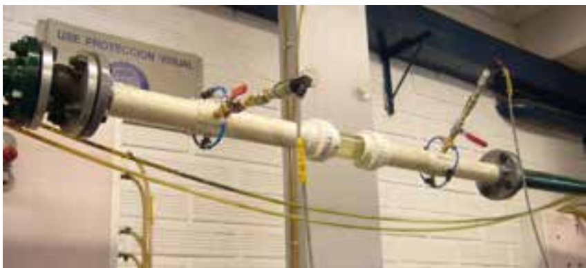
Figure 2. Flow system adapted for the permeability test
