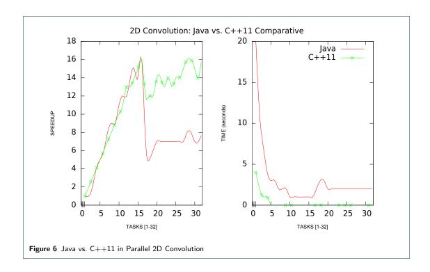
hundred iterations on data and, consequently, the synchronization overhead is much higher in the BZ–simulation than in the 2D convolution. In such case, the pool helps to improve the execution time obtained. With 2D-convolution implementations, to create a thread pool is not worthwhile, because it is very demanding in terms of runtime and then Java must pay a non rewarded price that finally affects program performance.
