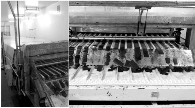
Figure 2. Solidification tunnel of Cocoa liquor
