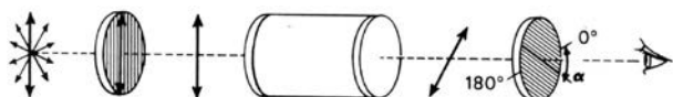
Figure 26. Measuring the concentration of a solution of sugar in the tube by means of rotation of polarized light.
