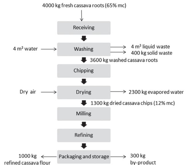
**Figure 1.** Mass balance of production of refined cassava flour.
