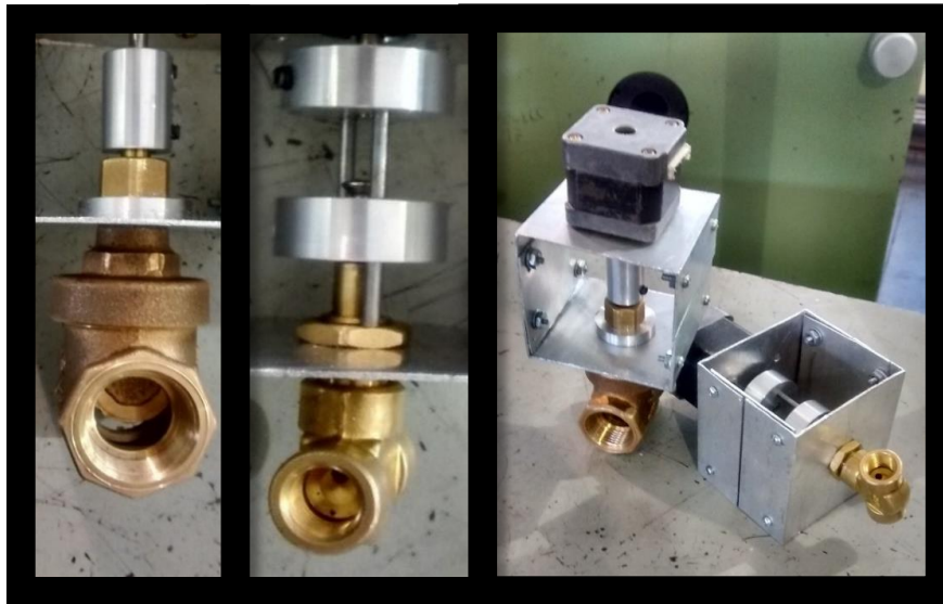
Figure 9 Machined bushings and supports. Left: Gate. Center: Needle. Right: Finished supports and couplings.
