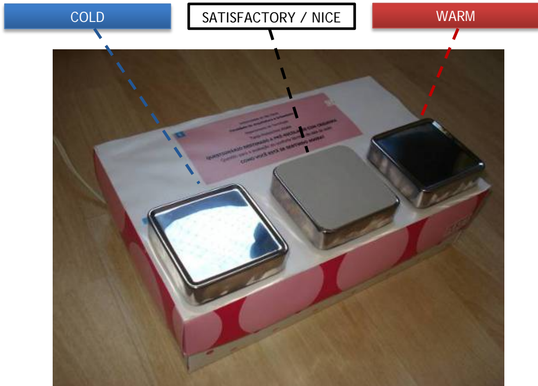
Figure 3. Tactile thermal model designed for questionnaires in environmental comfort surveys with blind children.
