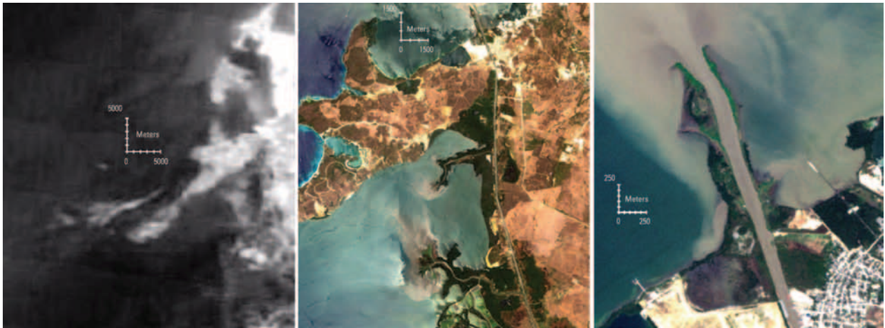
Figure 5. Comparative analysis of spatial resolution in the analysis of sediment in MODIS 250 m (left), Landsat 30 m (center) and RapidEye 5 m (right) images.
