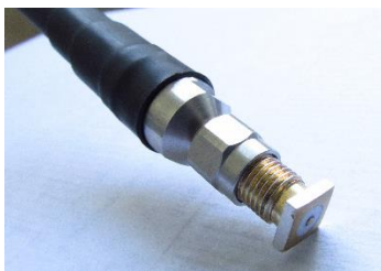
Figure 3 SMA probe used in the measurements.
