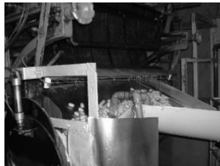
a) Cleaner to remove the coarse silk yarn spun b) Cocoons way out of the "shaken" cooker
