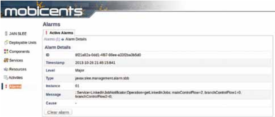
Figure 9. Alarm notification for QoS violation of LinkedIn-WS
