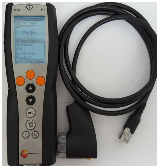
Figure 4 Exhaust gas analyzer equipment used (Source: Authors) 2.4 Estimation of polytropic coefficients
