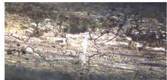
Figure 7. Steel core before exposure to the saline fog
