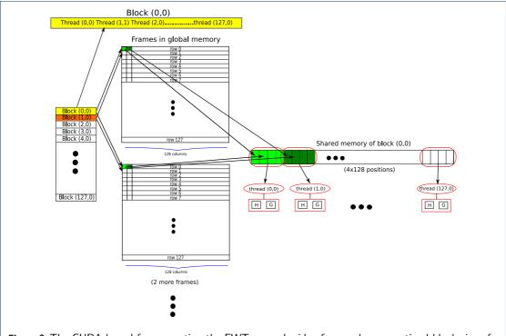
**Figure 2** The CUDA kernel for computing the FWT on each video frame when an optimal block size of 128 threads is used. The diagram is tailored to a frame size of 128x128 pixels, which forces a topology of 128x1 blocks for the grid. The i-th block loads 4x128 pixels into shared memory and computes 128 pixels for H and G, storing them in its i-th row.
