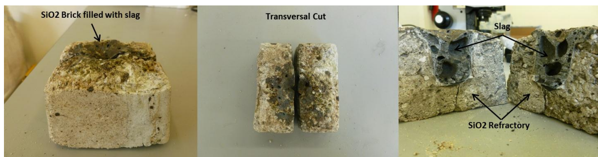
Fig. 6 Cup degradation laboratory test, \text{SiO}_2 brick filled with Slag-2.
