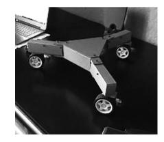
Figure 8. Physical model of the omni-directional mobile robot.
