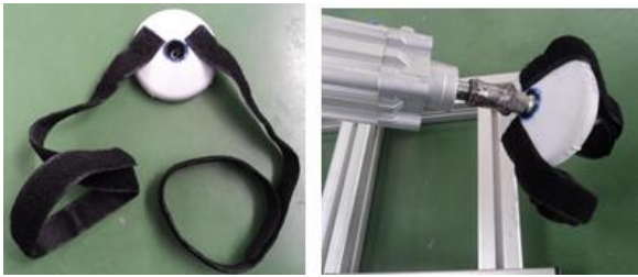
Figure 5. Left: rotating foot with cover; right: rotating foot attached to the brake pedal.
