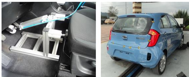
Figure 8. Test vehicle rear impact (KIA Picanto ION); left: mechanism mounted in the test vehicle; right: impact test.
