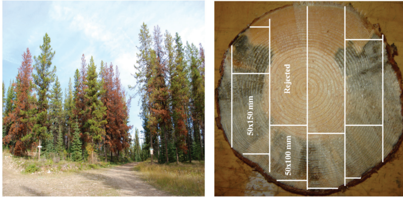
Figure 2. Targeted infected pine forest (reddish brown trees) in Kelowna, BC (left) and log cutting procedure aiming to maximize infected board output (right).
