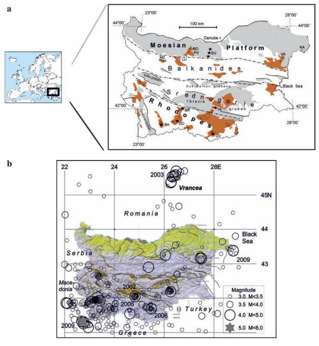
**FIGURE 1. a.** Main structural and tectonic units in Bulgaria (after van Hinsbergen *et al.*, 2008), **b.** Seismicity of Bulgaria (lower magnitude threshold 3.0, time period 2002-2011) on the background of Quaternary faults and Quaternary deposits (<a href="https://www.geology.bas.bg/geotech/Kvaternerni">https://www.geology.bas.bg/geotech/Kvaternerni</a> razlomi.jpg> 2012); the indicated years correspond to earthquakes mentioned in the text (all of them with M>4)
