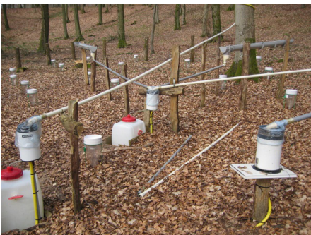
Figure 9-10. Throughfall and stemflow measurements
