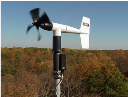
Figure 3. Anemometer and Wind Vane at 42 meters
