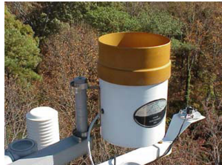
Figure 4. Temperature & Relative Humidity (left), rain (center) Solar Radiation (right) at 42 meters
