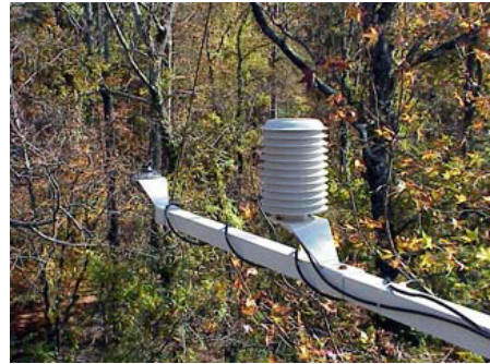
Figure 8. Temperature & Rel Humidity Cover (center) Solar Radiation (left) at 21 meters
