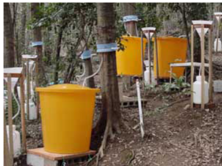
Figure 9-10. Throughfall and stemflow measurements
