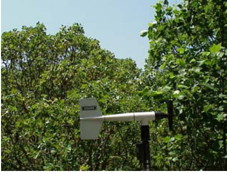
Figure 5. Anemometer and Wind Vane at 21 meters
