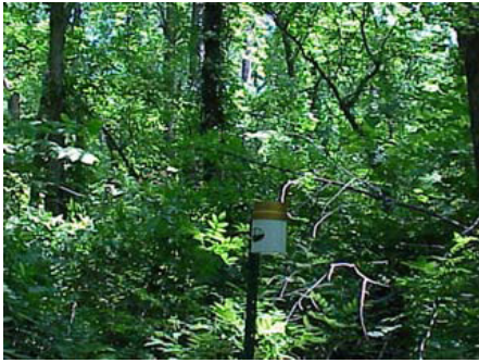
Figure 7. Under the Canopy Tipping Bucket Rain Guage
