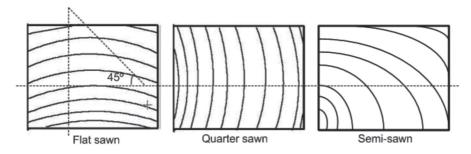
Figure 1. Determination of sawing pattern according to growth ring orientation on the end-grain section.
